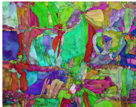
Figure 1. EBSD orientation map from additively manufactured 316L was collected at 6,700 ipps with Velocity Ultra with a 99% indexing success rate.
