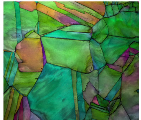
Figure 4. EBSD orientation map from deformed brass was collected at 2,000 ipps with Velocity Pro with a 99% indexing success rate.
